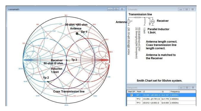
Shows that the receiver is matched. When the Antenna length is correct and the length of the coax transmission line is correct. For this type of Antenna matching system.
