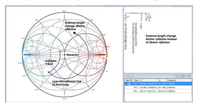
Shows when the Antenna element length is NOT correct. And the coax transmission line length is CORRECT. It is not on the matching circle. And is not on the road to matching with the receiver.
