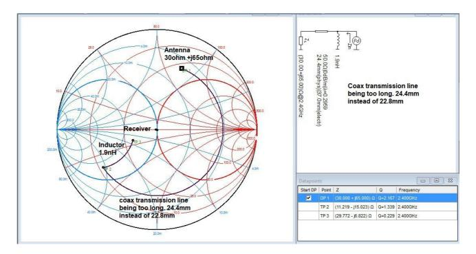
Shows when the Antenna element length is correct. But the coax transmission line is too long, and is not on the matching circle. And is not on the road to matching with the receiver.
