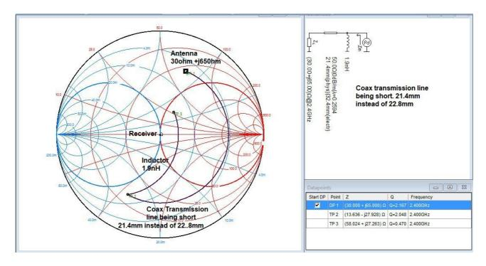
Shows when the Antenna element length is correct. But the coax transmission line is short and is not on the matching circle. And is not on the road to matching with the receiver.
