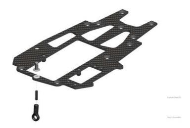
6. make 2 links as shown. The distance between the two balljoints should be 8.7mm
