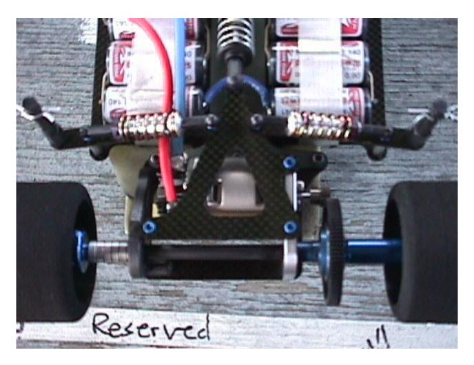
Next, take the 6 AE axle spacers you bought as "parts needed" and install them on the left-hand side. The end result is a rear axle spacing that is symmetrical to within .5 of a mm, or in other words, it's as close to center as I can measure it with the resources I have.
