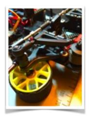
Front suspension. Now that the rear is good, we gotta get the front right! The most important thing with this is free movement of all components, and making sure the two sides are the same.
